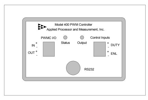
Figure 1.0-1 Model 400 PWM Controller.
