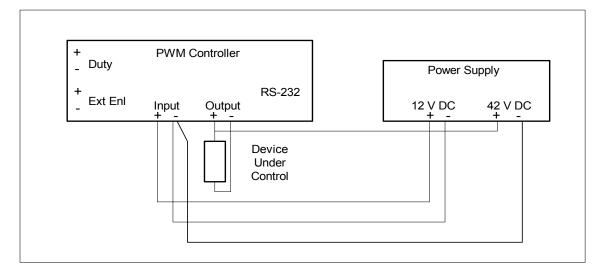
Figure 3.2-2 PWM Controller - Dual Supply Connection.
