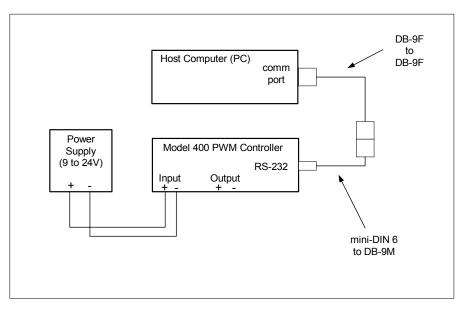
Figure 4.6-1. Recommended Set-up for PWM Controller Configuration
