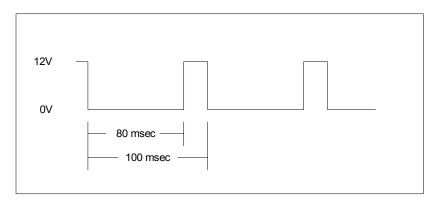
Figure 4.1.1-1 PWM Controller – Low Side Drive Output and Duty Cycle Definition.
