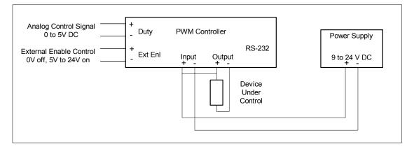
Figure 3.2-1 PWM Controller - Single Supply Connection.
