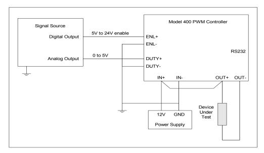
Figure 3.2-4 PWM Controller - Common Ground Connection.
