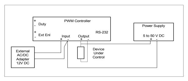
Figure 3.2-3 PWM Controller - Dual Supply Connection, using the kit adapter for PWMC power.
