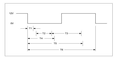
Figure 4.3-1. Analog Input Measurement Timing to the PWM Output Pulse Period (not to scale).
