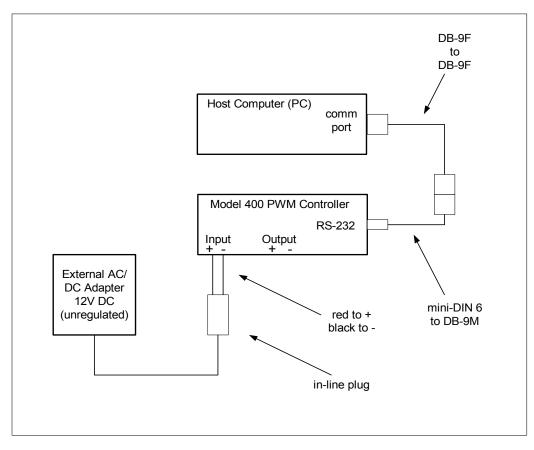
Figure 3.1-1 Model 400 PWM Controller – kit set-up.
