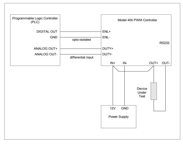
Figure 3.1-2 Model 400 PWM Controller – typical installation.
