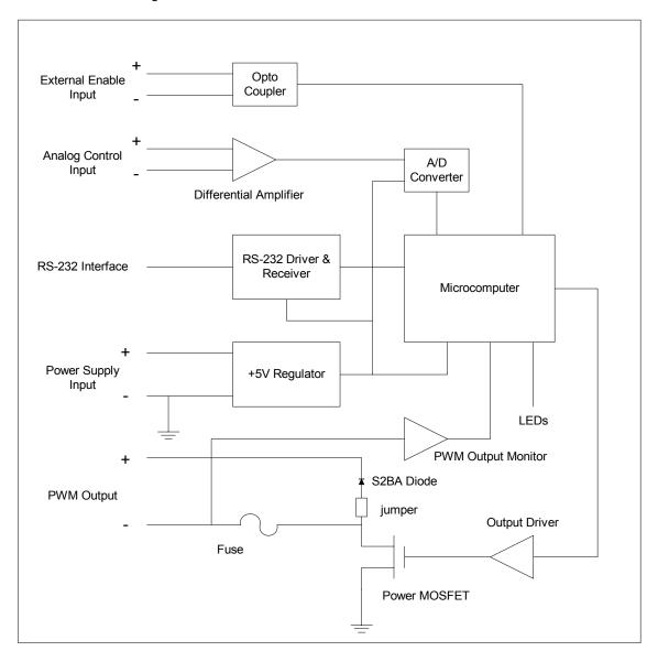
Figure 4.1-1 Model 400 PWM Driver / Controller - Block Diagram.
