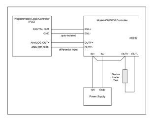
Once power is applied to the PWMC 400, the unit will operate as configured (analog or RS-232 to PWM duty cycle out).
