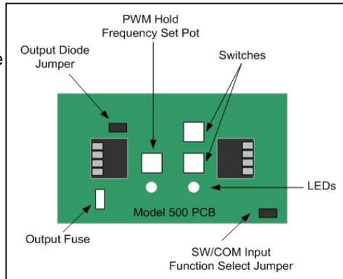
The SW/COM jumper is used to set the function of the SW/COM contact input. With the jumper removed (factory default), the input acts as another output trigger. With the jumper installed, the input acts as a PWM hold disable. When in PWM hold disable mode, the SW/COM input may be used to dynamically override the PWM hold function and force full-on at the output when required for high load conditions.
